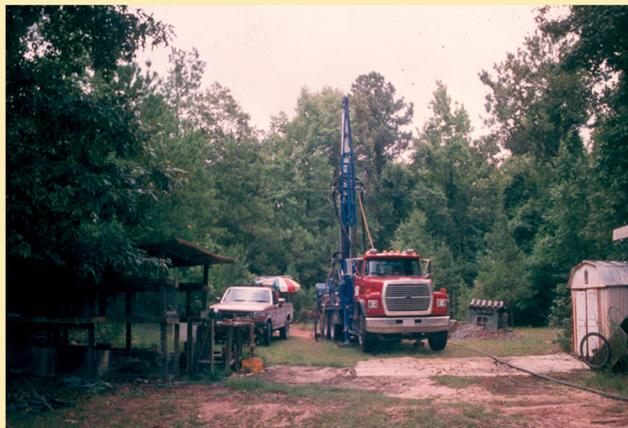
Vulcan Materials drill rig at Mr. Schroeder's home in Wetumpka. Drilling to ~ 300 m occurred from June 24 to July 18, 1998. We now refer to this as A.U. Scientific Borehole #98-01. The drill core from this well was studied by Reuben C. Johnson for his M.S. thesis (2007); and by us for our 2002 *EPSL* paper.
