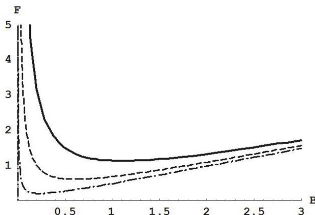
Fig. 2. Plot of the function  $F(A, B)$  representing the dependence of the monopole contribution to the width  $w_{nl \rightarrow 1s}^{(0)}$  (from Eq. (14) on the scaled dimensionless electron velocity  $B$  (defined in Eq. (13)) for three values of the parameter  $A$ :  $A = 1$  (solid line),  $A = 0.5$  (dashed line), and  $A = 0.25$  (dash-dotted line). The function  $F(A, B)$  is defined by Eqs. (15), (16).
