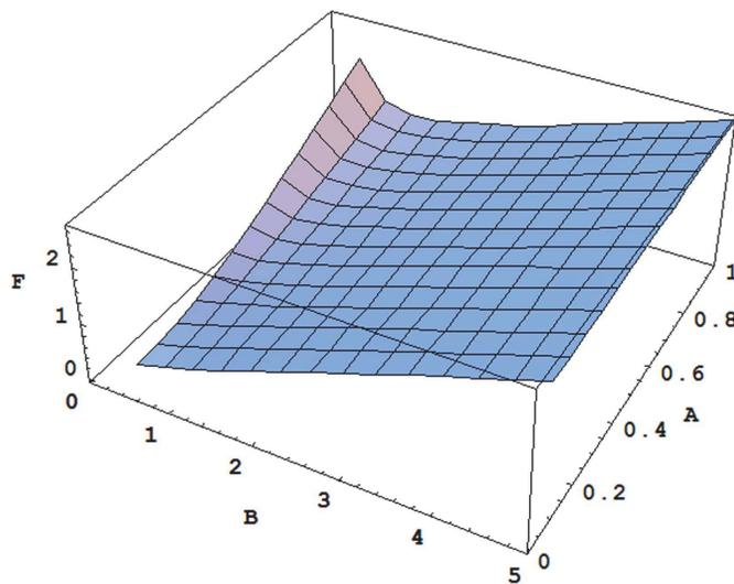
**Fig. 1.** Three-dimensional plot of the function  $F(A, B)$  representing the dependence of the monopole contribution to the width  $w^{(0)}_{nl \rightarrow 1s}$  (from Eq. (14)) on the scaled dimensionless electron velocity B (defined in Eq. (13)). The function  $F(A, B)$  is defined by Eqs. (15), (16).
