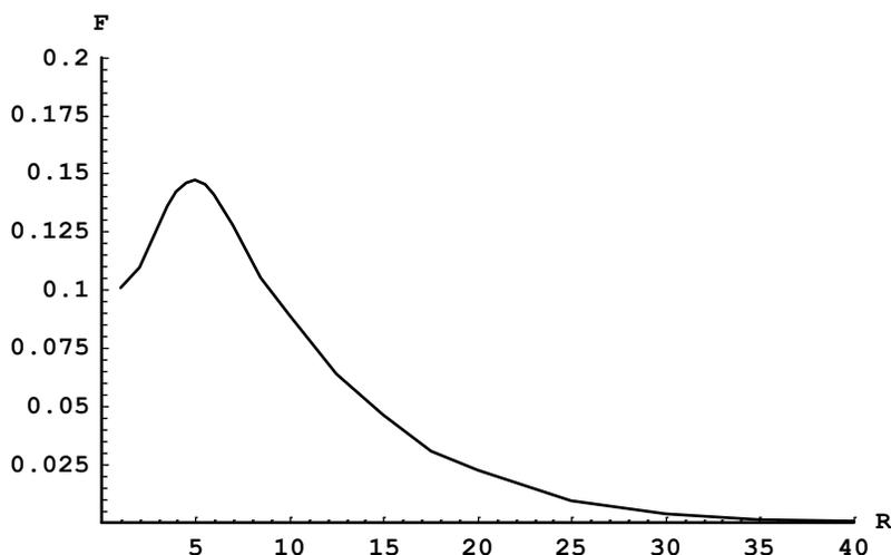
Fig. 2. The frequency  $F$  (in units of  $10^5 \text{ cm}^{-1}$ ) of the radiative transitions between these two terms from Fig. 1 versus the internuclear distance  $R$  (in atomic units).
