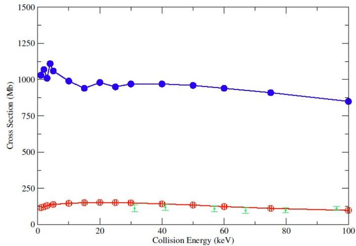
**Figure 1. Single Ionization of H. Solid blue circles: TDCC for anti-alpha particle, striped red circles: TDCC for antiproton particle, error bar circles: Experiment for antiproton particle ( $1.0 \text{ Mb} = 1.0 \times 10^{-18} \text{ cm}^2$ ).**
