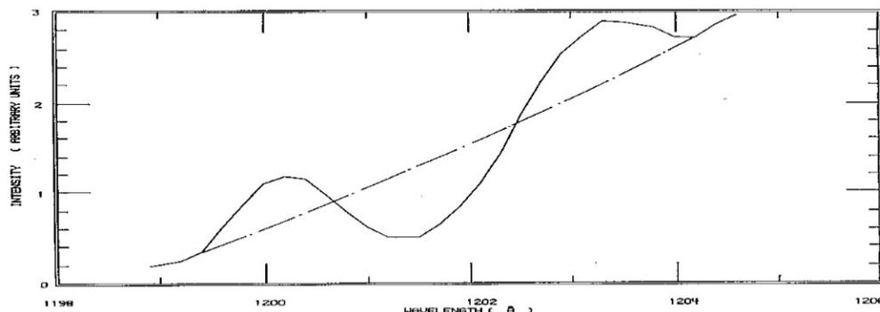
Fig. 2. A magnified part of the profile of the Ly-alpha line, obtained in the high-precision, benchmark experiment at the gas-liner pinch [6], showing the observed bump-dip-bump structure.
