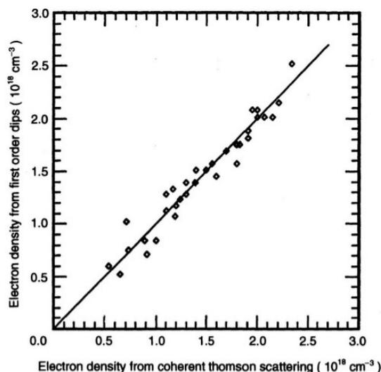
Fig. 3. Electron densities, obtained from the experimental positions of the Langmuir-wave-caused bump-dip-bump structures versus the electron densities measured by the coherent Thomson scattering. The comparison is shown at many electron densities in the experiments at the gas-liner pinch [6].
