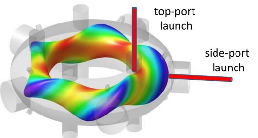
**I. Launch through side-port into radial B-gradient**
