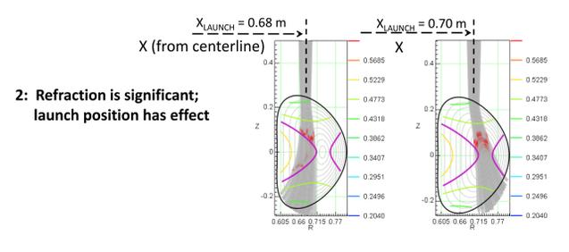
**3: Top-launched beams will undergo greater refraction due to the non-normal incident angle, and may limit effective heating to density  $n_{e0} \leq 0.3 \times 10^{19}$  m<sup>-3</sup>.**
