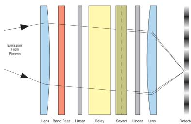
**Collection Lens:** collimates plasma emission from a wide angle into the diagnostic
