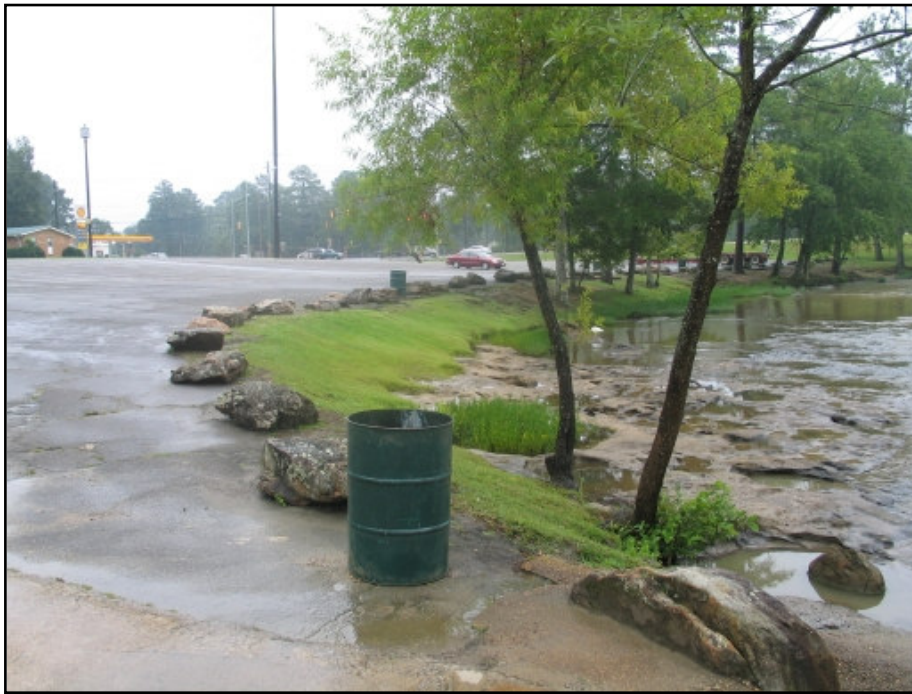
Inadequate vegetated buffer strip between Noccalula Falls parking lot and Black Creek
