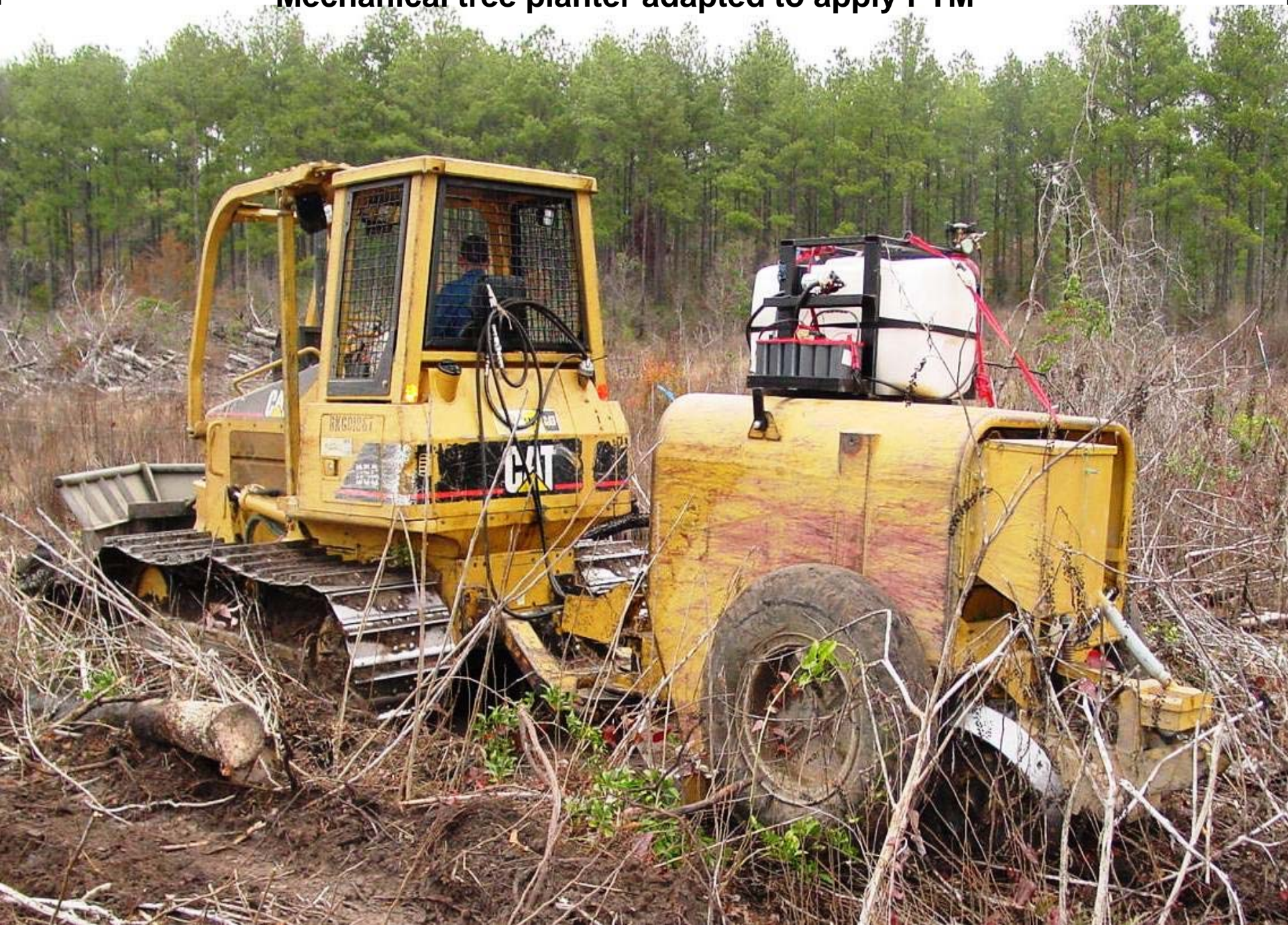
Mechanical tree planter adapted to apply PTM
