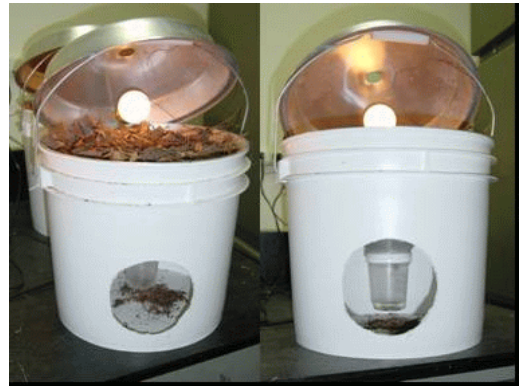
Figure 2.6. Berlese funnel with ethanol filled collection cup used to extract insect from duff sample.
