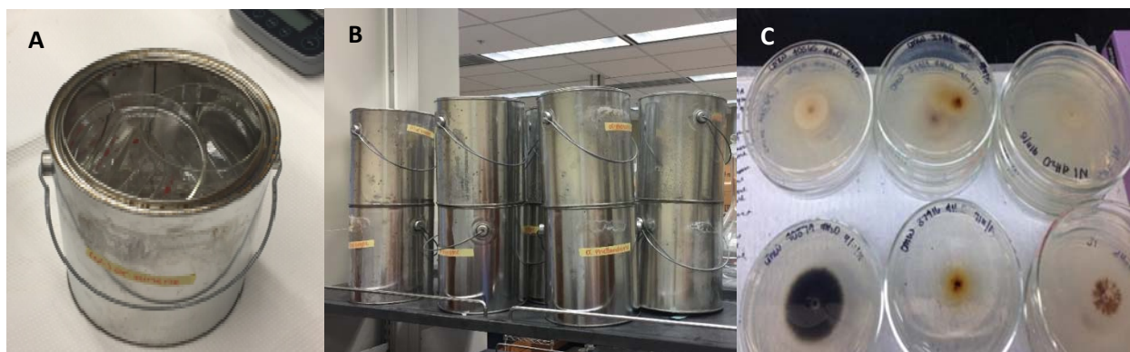
Figure 4.3. Glass plates inoculated with Amylostereum spp. were stacked inside paint cans (A) to create atmospheric chambers (B). After the 7 day growth period was completed, plates were removed from paint can chambers (C). The leading edge of hyphae was traced after the seventh day of treatment.
