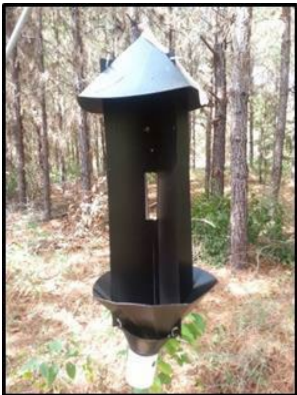
Figure 3.4. A panel trap to be baited with hanging vials of 3-carene and 95% ethanol.
