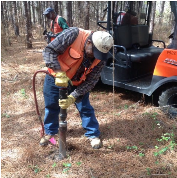
Figure 2.5. Pneumatic soil core sampler with a plastic tube inside it used to collect soil cores.
