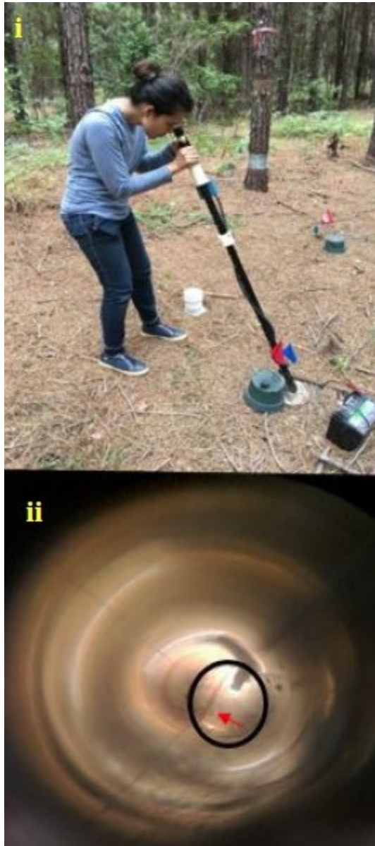
Figure 3.8. (i) Observing root intersections with an optical periscope e. The black rectangular object on the ground is a battery which is connected to the periscope to power the light, (ii) the faint line noted by the red arrow is a new root.
