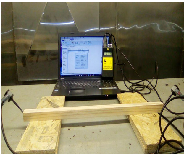
Fig. 1 Setup for the estimation of the acoustic velocity using Microsecond Time
