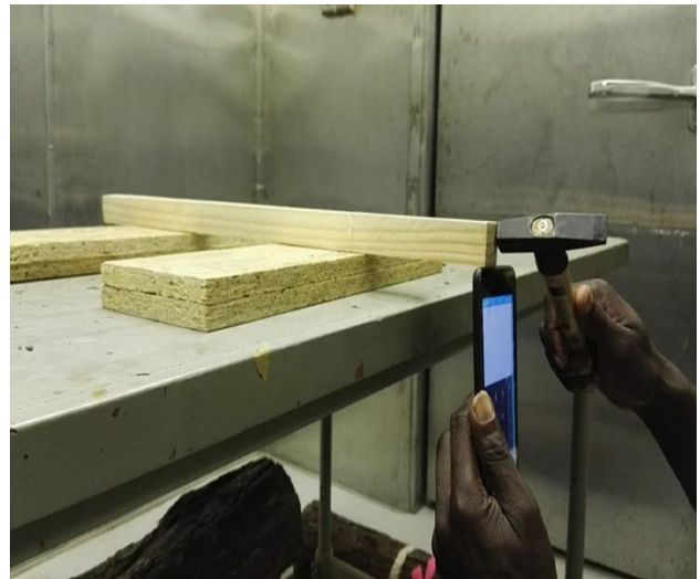
Fig. 2 Setup for the estimation of acoustic velocity using resonance log grader
