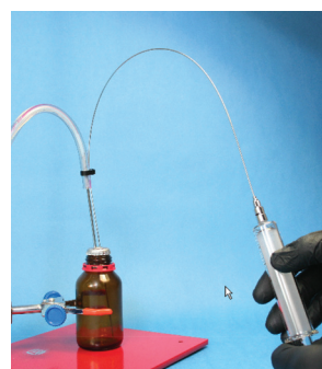
Fig. 8 Filling syringe using nitrogen pressure
