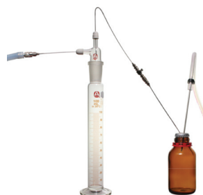
Fig. 12 Double-tipped needle transfer to graduated cylinder
