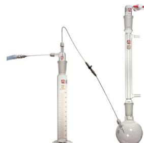
Fig. 13 Double-ended needle transfer with syringe valve
