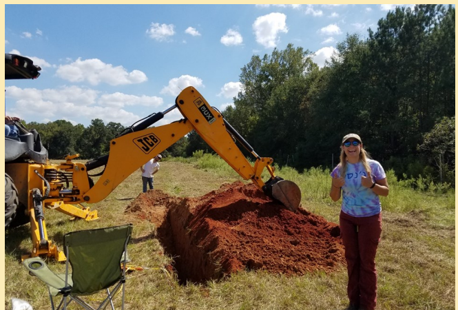
Mike Salisbury and Sam Eckes getting a little help from a back hoe to dig a trench for a GPR buried objects experiment at the EV Smith Experimental Farm.
