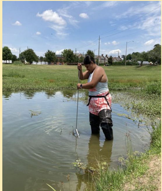
Sophia Saucedo, practicing using a depth integrated water sampler for measuring Total Suspended Solids in the pond at Ag Heritage Park.
