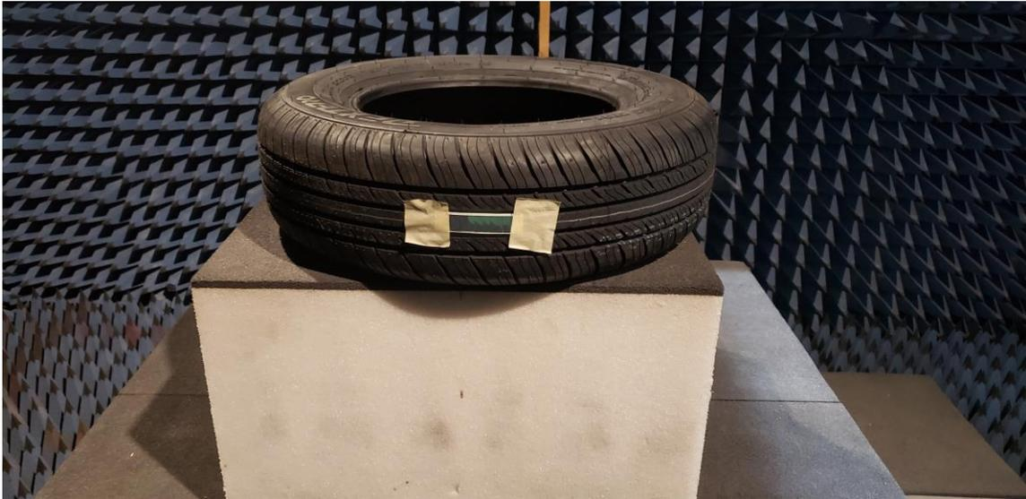
**Figure 2: Position of Tag on Tire**
