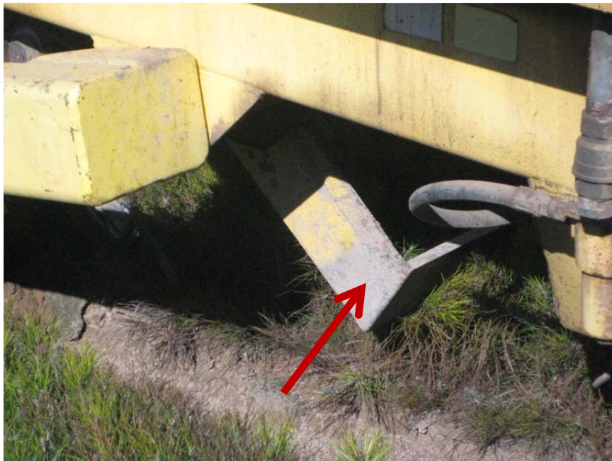
Figure 1. Love full-bed lifter seedling lifter bar in raised (unused) position.
